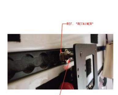
5. The VRS Should Now be Fully Engaged and Locked in the Aircraft Seat Tracks.
